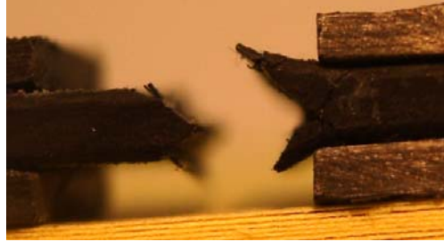
Figure.1. Matrix/Inter-fibre failure in carbon fibre specimens tested under transverse compression.
