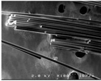
Figure 7: Micrograph showing a group of fiber failures after static fatigue at 1000°C, under a stress of 250 MPa during 13 days.
