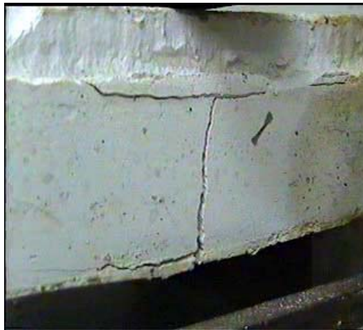
Figure 7: The crack occurred after the middle layer fails in laminated composite panel.
