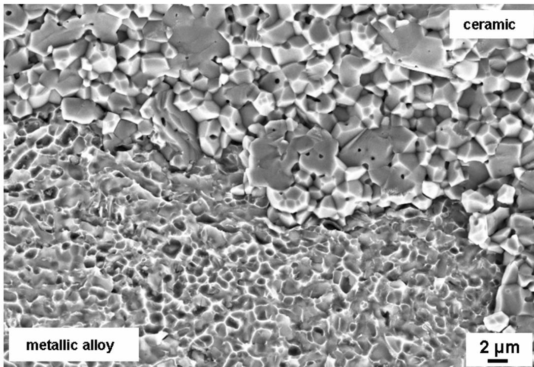
Figure 7: SEM micrograph showing the interfacial region
