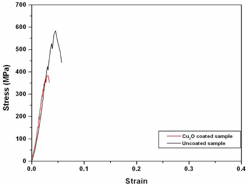
Figure 5: Stress-strain curve for single domain samples compressed along the freezing direction
