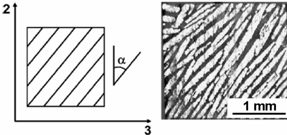
Figure 2: Definition of the angle  $\alpha$ , marking the orientation of a single domain composite specimen with respect to direction 2 of the specimen coordinate system [13]
