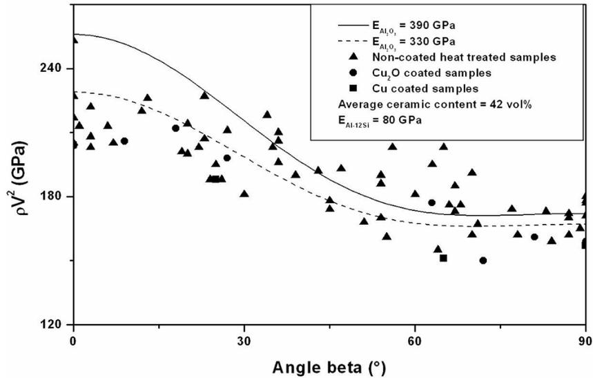
Figure 4: Effect of domain orientation on the quantity  $\rho V^2$  for single domain samples
