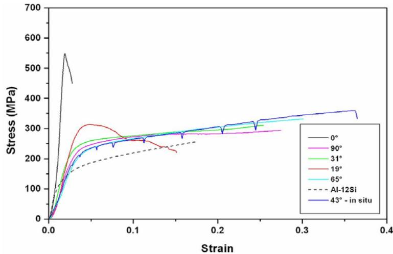
Figure 8: Compressive stress-strain plot for single domain samples compressed transverse to the freezing direction: effect of domain orientation
