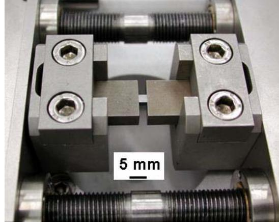
Figure 3: Single domain sample placed between two flat punches in the miniature mechanical test device
