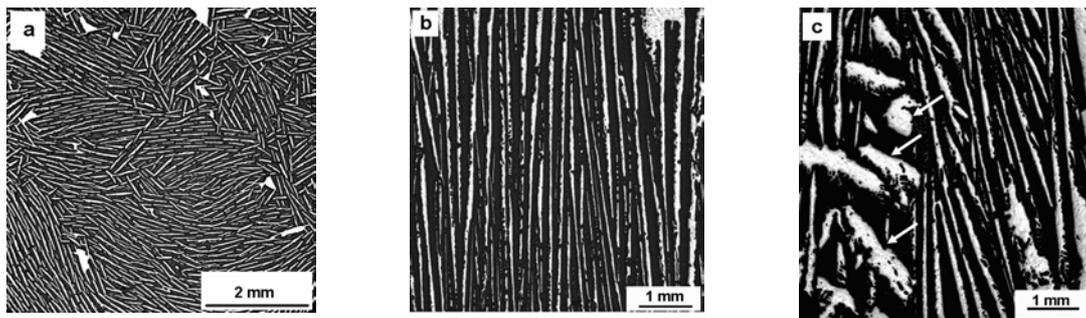
Figure 1: Microstructures of the three orthogonal faces of the composite; (a) face perpendicular to freezing direction and (b - c) faces parallel to the freezing direction
