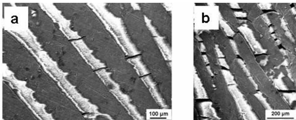
Figure 9: SEM micrographs showing the damage evolution when compressed at  $43^\circ$  to the domain orientation in a single domain uncoated sample (Compressive loading in horizontal direction); (a) initial transverse cracking within the ceramic lamellae, (b) extensive transverse cracking of the ceramic lamellae and ductile cracking of the metallic alloy at a much higher total strain
