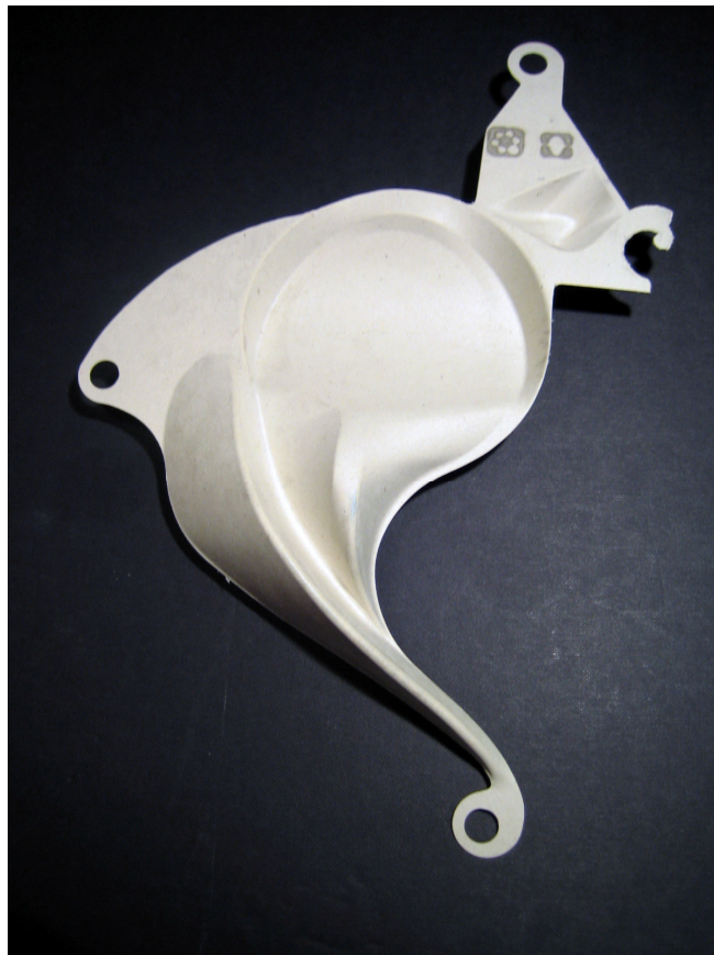
Figure 3: A ‘kofes’ moulded in 75% CTMP pulp fibre and 25% PLA. The material is fully renewable. Design: Farvash Razavi and Nandi Nobell.
