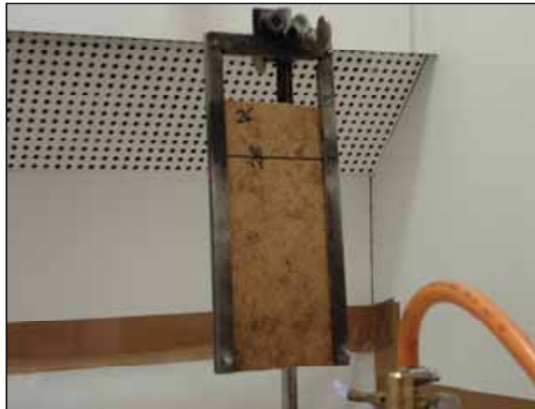
Figure 10: Natural fiber composite by fire testing
