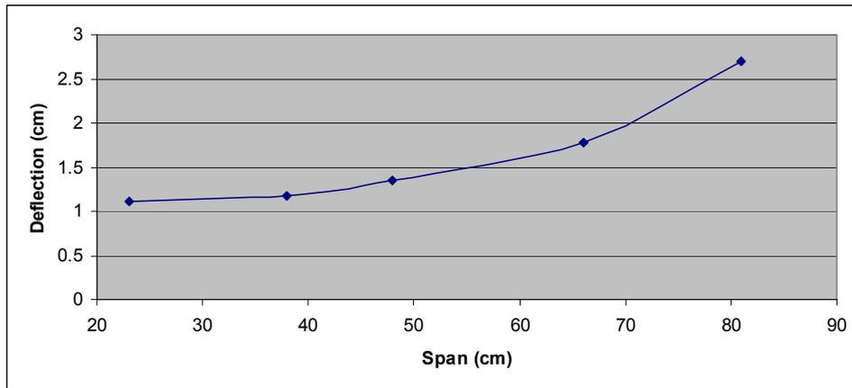
Figure 9: Deflection vs. Span for composite sandwich beam.
