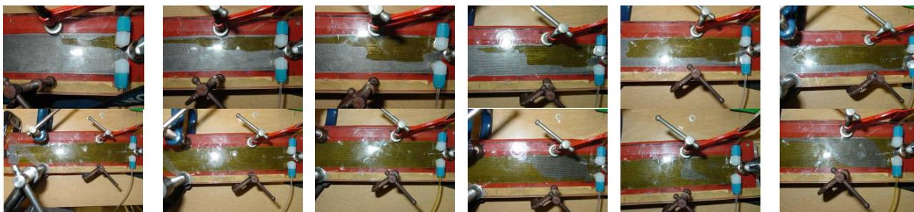
Figure 6: Flow behaviour of solution with silicon gasket sealing material. (Photos taken sequentially from left to right).
