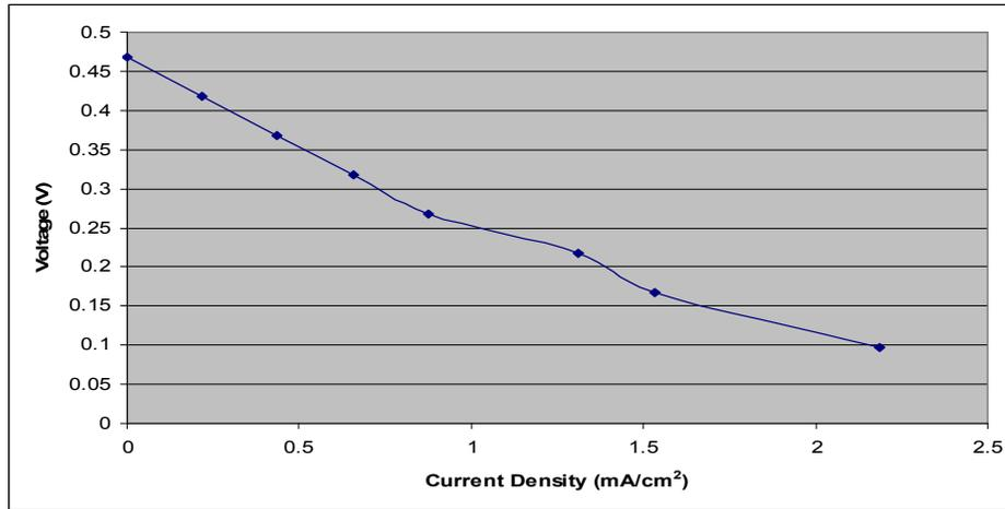
Figure 5: Polarization curve for pultruded fuel cell
