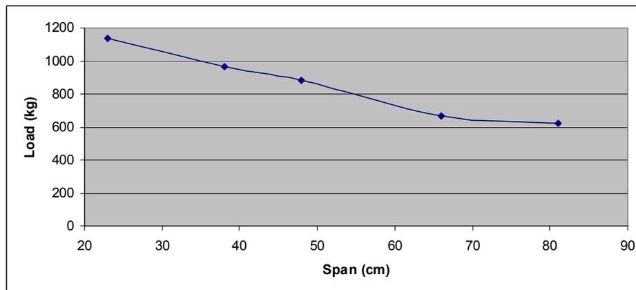
Figure 8: Load vs. Span for composite sandwich beam.
