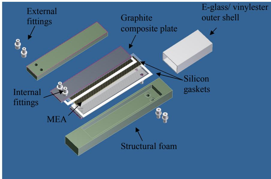
Figure 1: Schematic of pultruded, structural fuel cell
