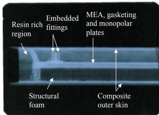
Fig. 2: Radiograph (view from side) of pultruded fuel cell beam.
