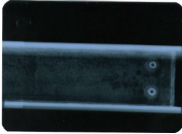
Fig. 3: Radiograph (view from top) of the pultruded fuel cell beam.
