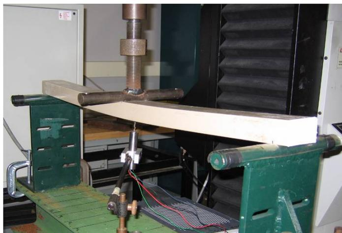
Figure 4: Sandwich beam undergoing flexure test
