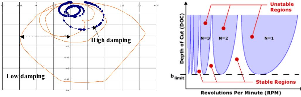
Figure 1: Stability of a cutting process
