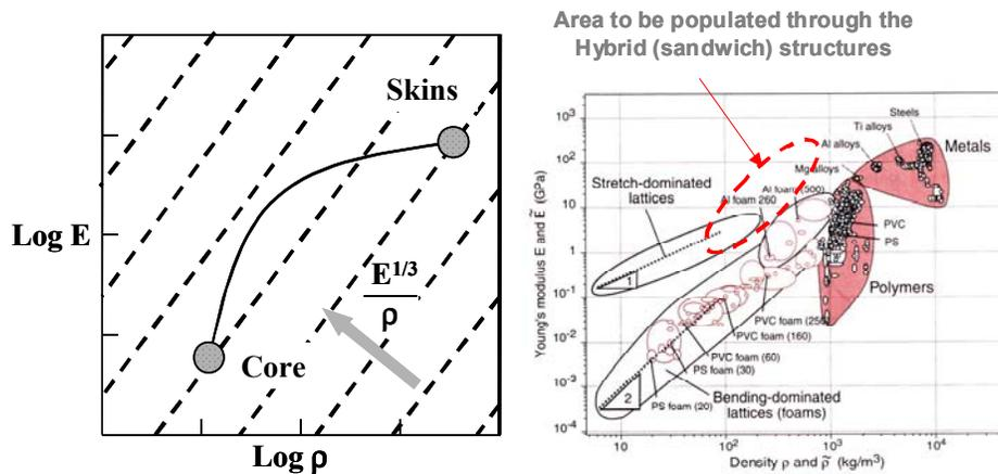
Figure 4: Structural index of sandwich panels
