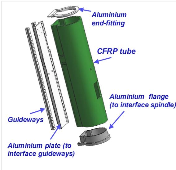
Fig. 8: Machine tools part (ram) made in CFRP with metallic end-fittings
