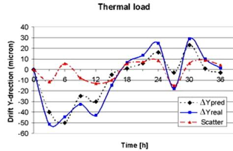
Figure 11: Test results - actual tool tip displacement vs. predicted one.
