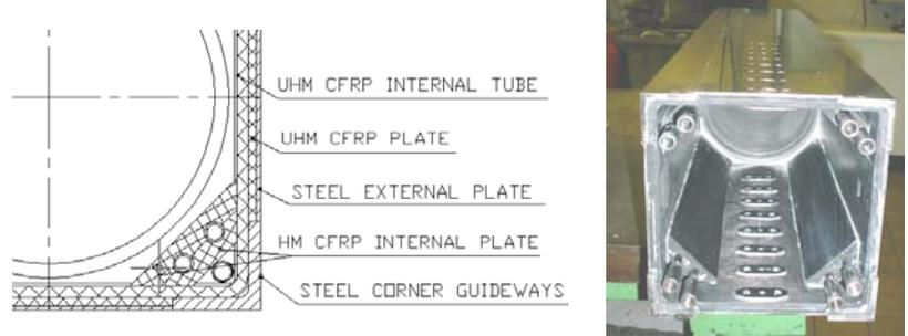
Figure 7: Ram cross section - Ultra high speed module
