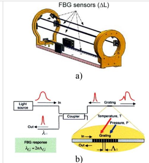
Fig. 9: a) Ram with FBGs sensors
