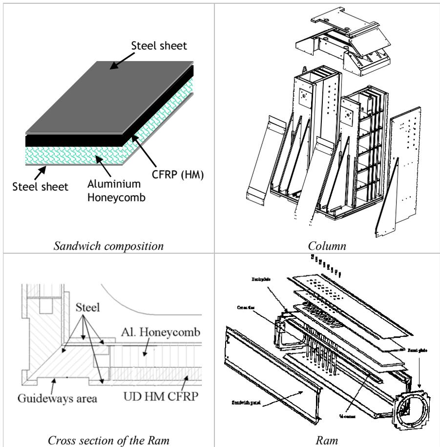
Figure 6: Sandwich hybrid material and applications
