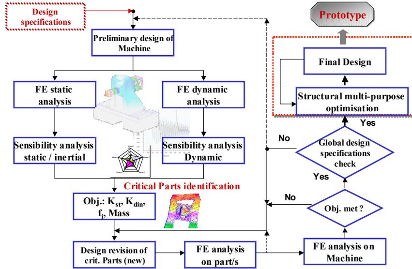
Figure 5: The FE design flowchart
