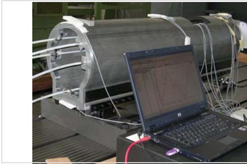
Figure 10: Test-bench setup of Ram with FBG sensors
