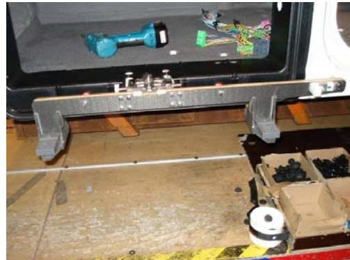
Figure 15 A manual fixture designed in composite material
