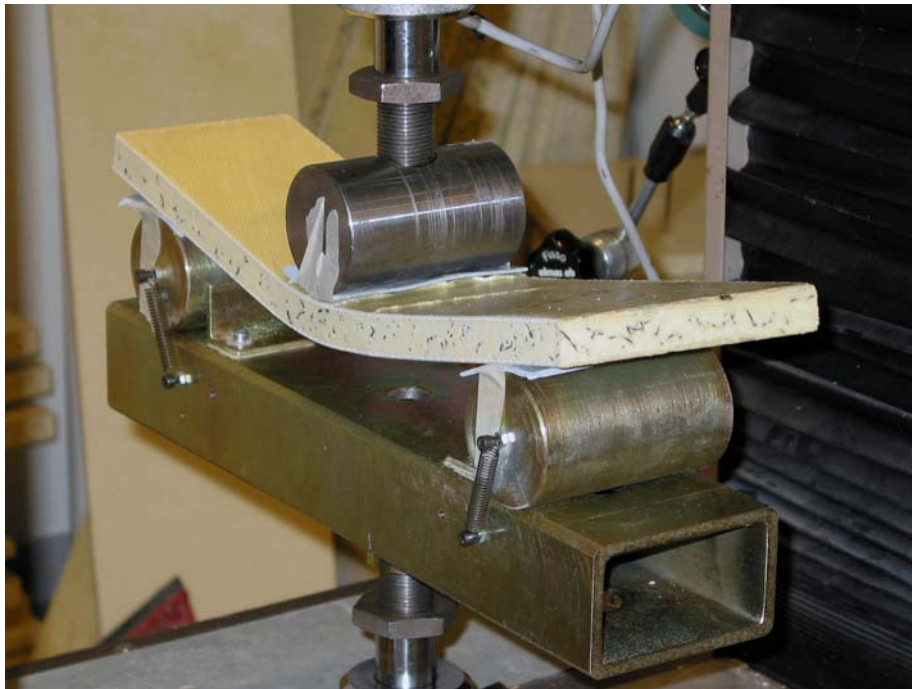
Figure 8: 3-point bending testing according to EN ISO 141 25 – Fibre reinforced plastic composites – Determination of flexural properties.
