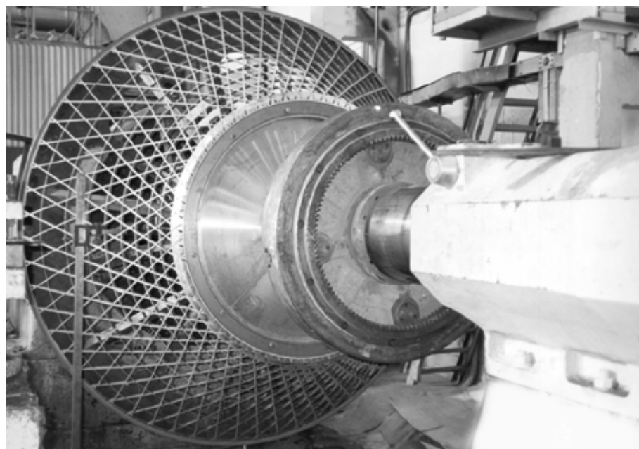
Figure 5. Machining of the lattice adapter
