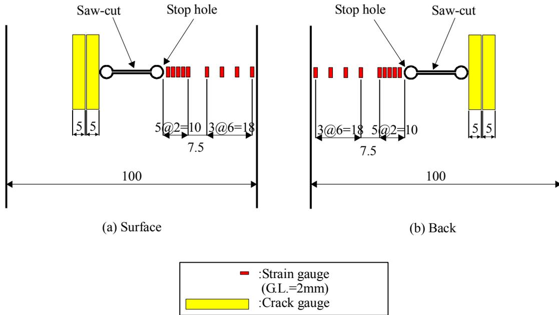
Fig.-2 Position of gauges
