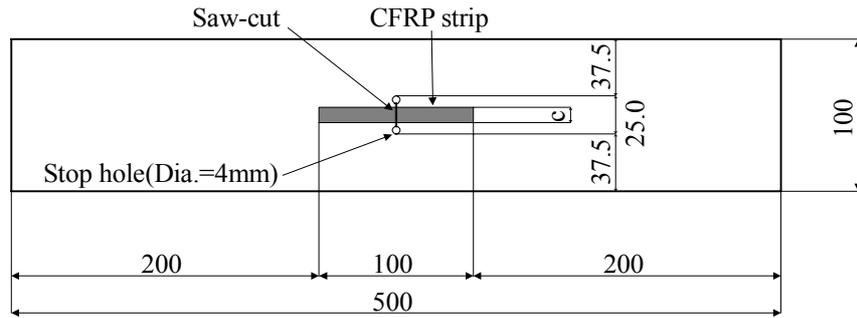
Fig.-1 Specimen configuration
