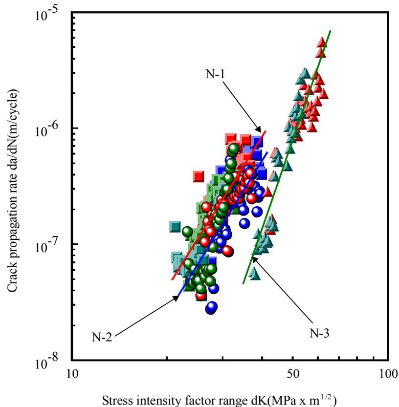
Fig.-5 Relation between crack propagation rate and stress intensity factor range
