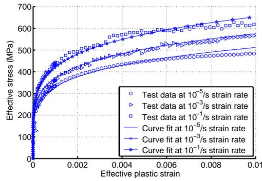
“Fig. 16. Effective stress – effective plastic strain curves at various strain rates.”
