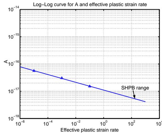
“Fig. 17. Log-log plot for the rate-dependent amplitude A.”
