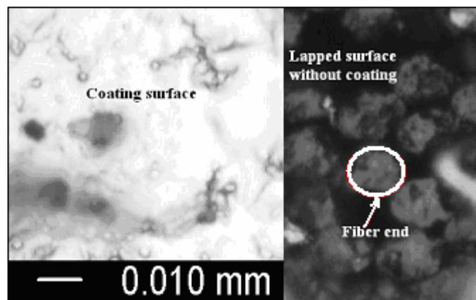
“Fig. 2. Micrographs showing fiber ends in specimens with coating and without coating
