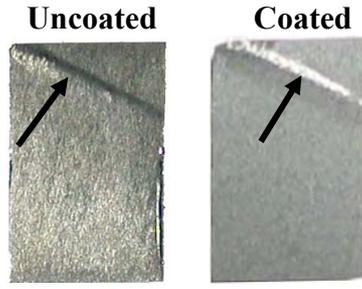
“Fig. 8. Microbuckling failure mode in 15° coated and uncoated specimens at 10<sup>-5</sup>/s strain rate.”
