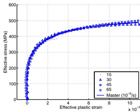
“Fig. 13. Collapsed effective stress – effective plastic strain curves for AS4/3501-6 carbon fiber composite at strain rate  $10^{-5}/s$  with  $a_{66}=7.0$ .”
