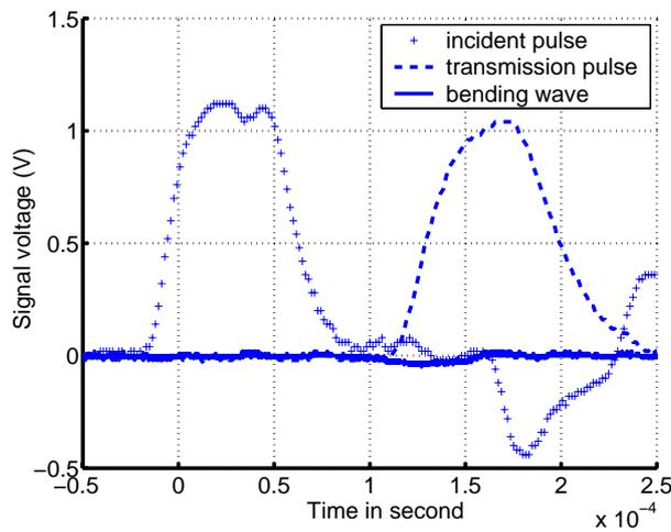
“Fig. 6. Strain histories picked up by strain gages at locations A, C, and D in 15° off-axis AS4/3501-6 composite specimen coated with titanium and tested with lubricant.”
