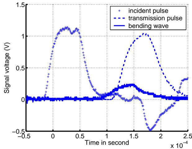
“Fig. 5. Strain histories picked up by strain gages at locations A, C, and D in lapped 15° off-axis AS4/3501-6 composite specimen with lubricant.”
