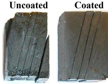
“Fig. 9. Matrix shear failure for 15° coated and uncoated specimens at strain rates higher than 10<sup>-1</sup>/s.”
