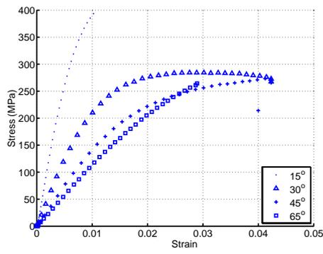
“Fig. 12. Stress strain curves at  $10^{-1}/s$  strain rate.”
