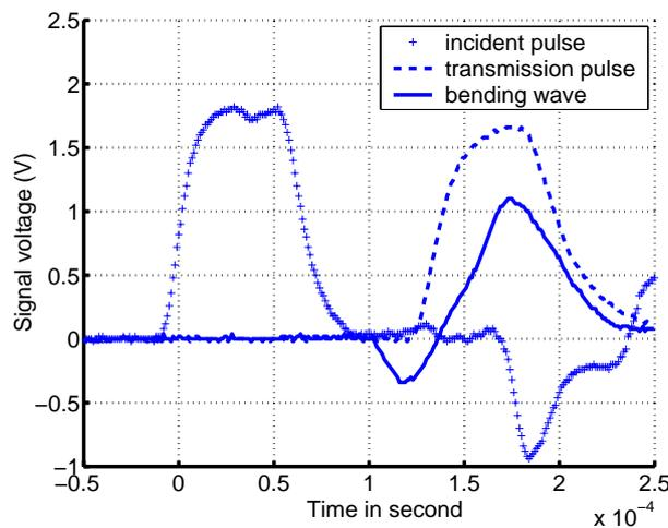
“Fig. 4. Strain histories picked up by strain gages at locations A, C, and D in lapped 15° off-axis AS4/3501-6 composite specimen w/o lubricant.”
