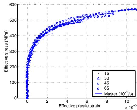
“Fig. 14. Collapsed effective stress – effective plastic strain curves for AS4/3501-6 carbon fiber composite at strain rate  $10^{-3}/s$  with  $a_{66}=7.0$ .”
