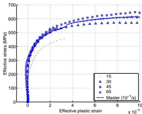
“Fig. 15. Collapsed effective stress – effective plastic strain curves for AS4/3501-6 carbon fiber composite at strain rate  $10^{-1}/s$  with  $a_{66}=7.0$ .”
