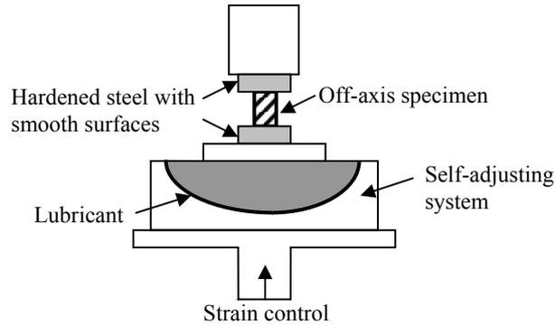
“Fig. 7. Schematic of compression test with self-adjusting system.”
