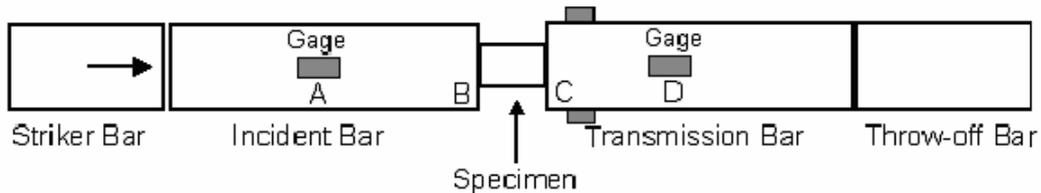
“Fig. 3. Schematic of Split Hopkinson Pressure Bar.”
