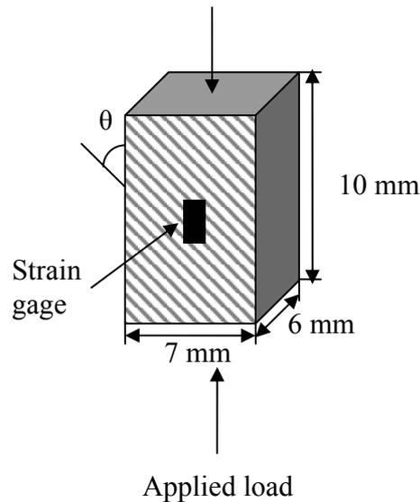
“Fig. 1. Small brick off-axis specimen with off-axis angle  $\theta$ .”
