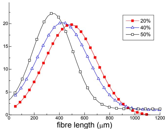
**Fig. 10.** Fibers length distribution for different fibers content values.
