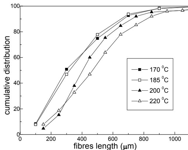
Fig. 4. Cumulative distribution of fibers length versus chamber temperature.
