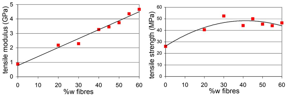
Fig. 6. Effects of fibers content on tensile properties.
