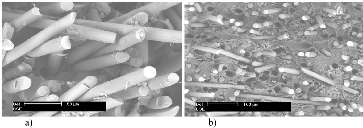
**Fig. 7.** SEM images: a) 55%w of fibers; b) 45%w of fibers.
