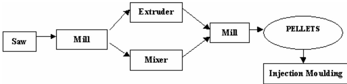
Fig. 1. Recycling procedure scheme.
