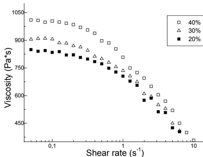
Fig. 11. Viscosity curves for different fibers content values.
