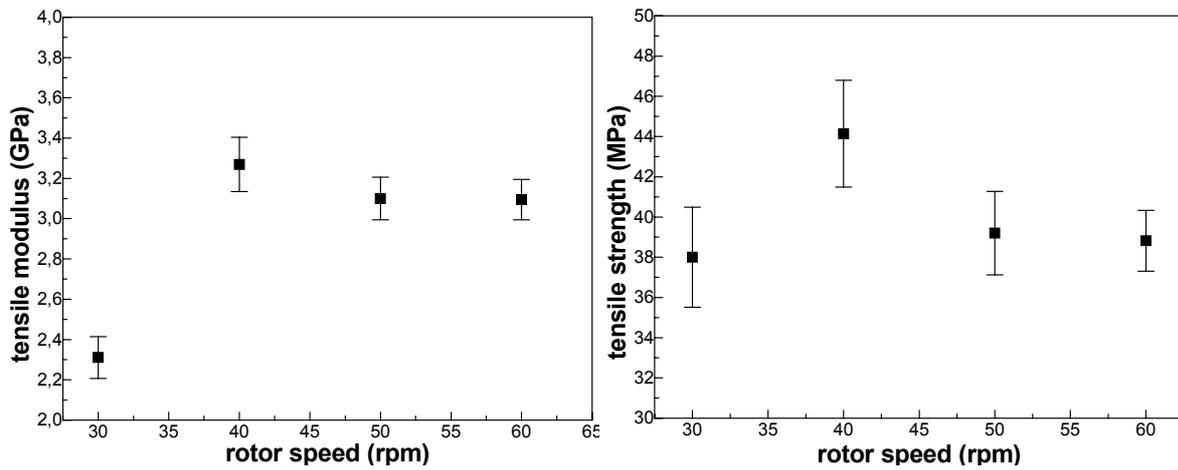
Fig. 5. Effects of rotor speed on tensile properties.
