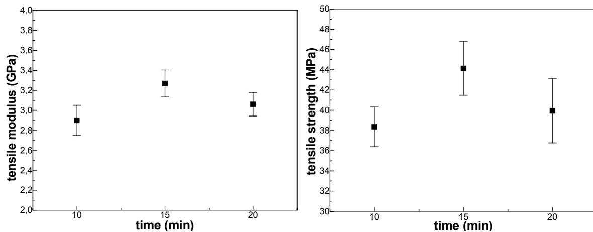
Fig. 2. Effects of mixing time on tensile properties.
