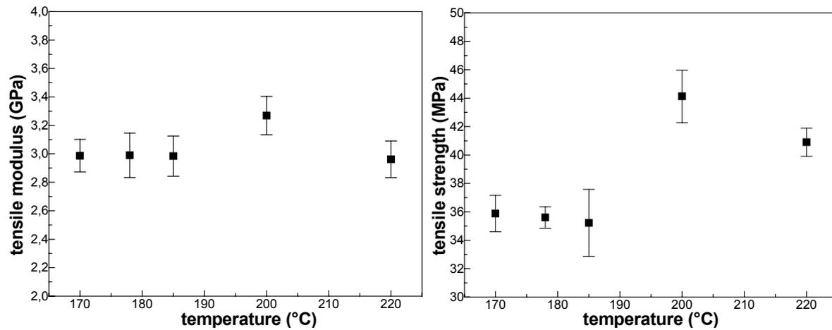
Fig. 3. Effects of chamber temperature on tensile properties.
