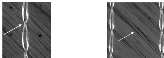
Figure 1. Top view of a [-45/+45] NCF showing a) the thread and b) the crossings.
