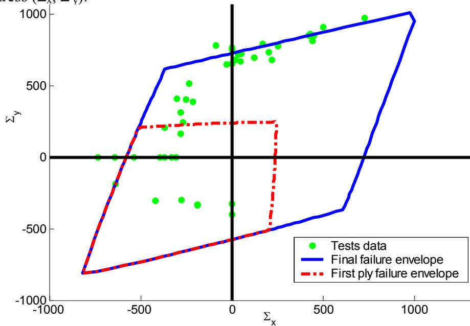
**Fig. 11** : Failure envelope of quasi-isotropic laminate in AS4/3501-6 Epoxy
