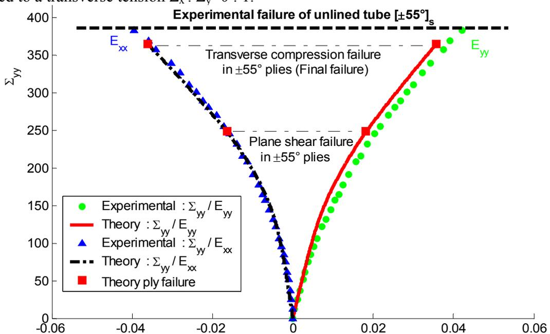
Fig. 10 : Behavior of  $[\pm 55]_s$  laminate in Elass/MY750 Epoxy
