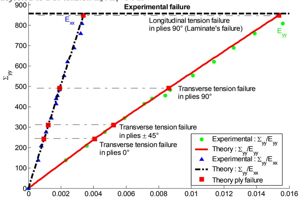
Fig. 9 : Behavior of Quasi-isotropic laminate in AS4/3501-6 Epoxy
