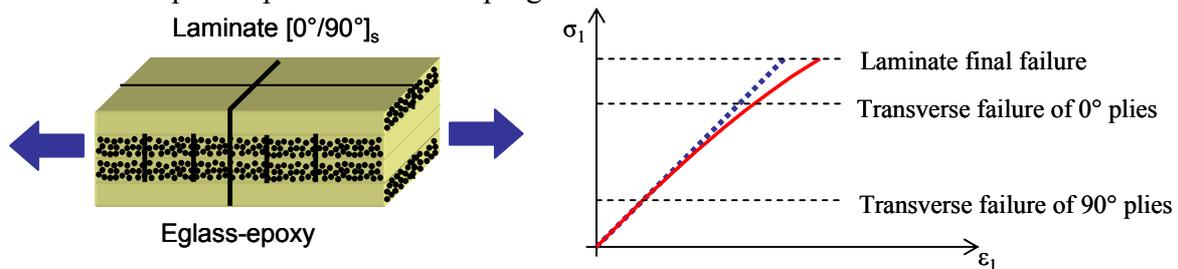
Fig. 2 : Progressivism of laminate's failure
