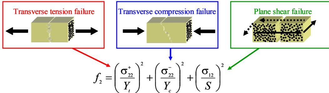
Fig. 6 : Interfiber failure mode
