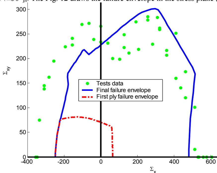
**Fig. 12** : Failure envelope of  $[90^\circ/\pm 30^\circ]_s$  laminate in E-glass/LY556
