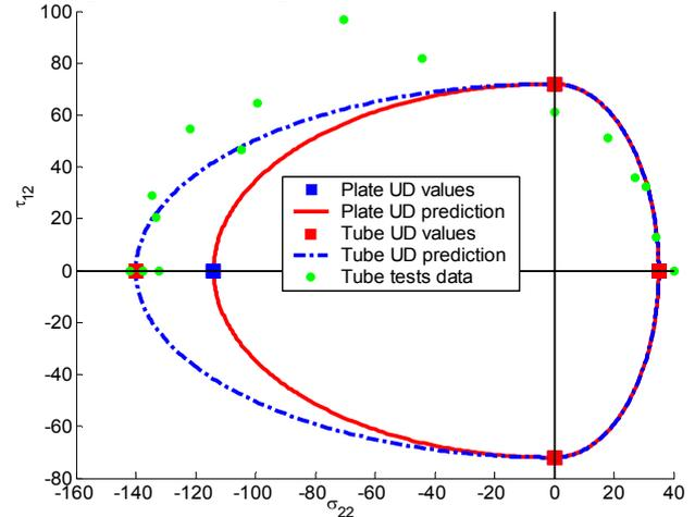
Fig. 8 : Failure envelope of UD in E-Glass/LY556
