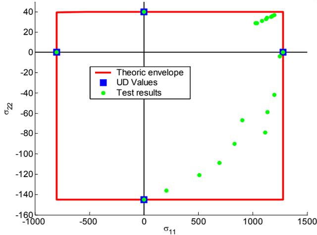
Fig. 7 : Failure envelope of UD in E-glass/MY750
