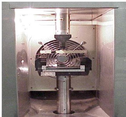
**Fig.2.** Three-point bend test conducted within an environmental test chamber
