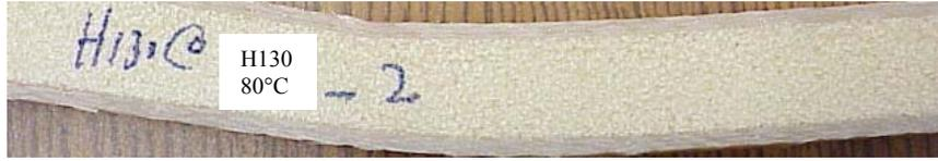
**Fig.5.** Plastically strained H130 beam after quasi-static test at 80°C
