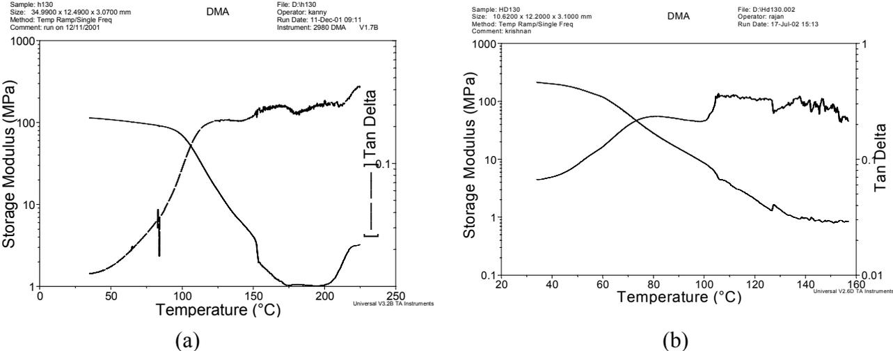
**Fig.3.**  $E'$  and  $\tan\delta$  as a function of temperature for (a) H and (b) HD foams, DMTA 3 point bending (1 Hz, 2°/min)
