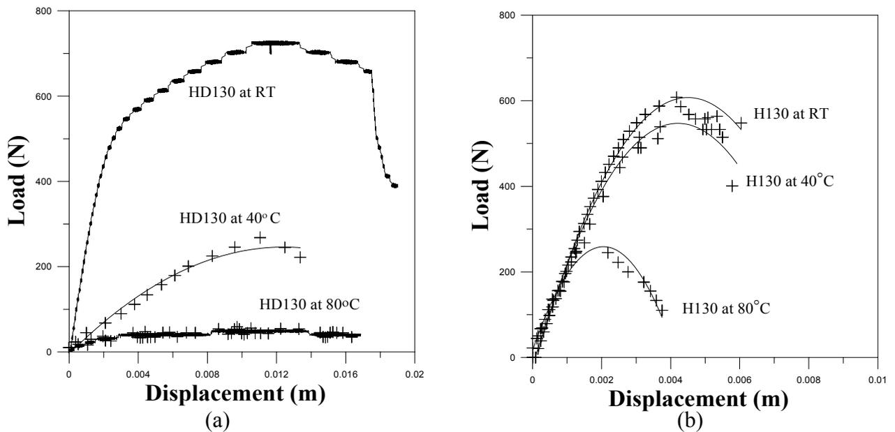
**Fig.4.** Load-displacement curves at RT, 40 and 80°C for (a) HD and (b) H sandwich structures.
