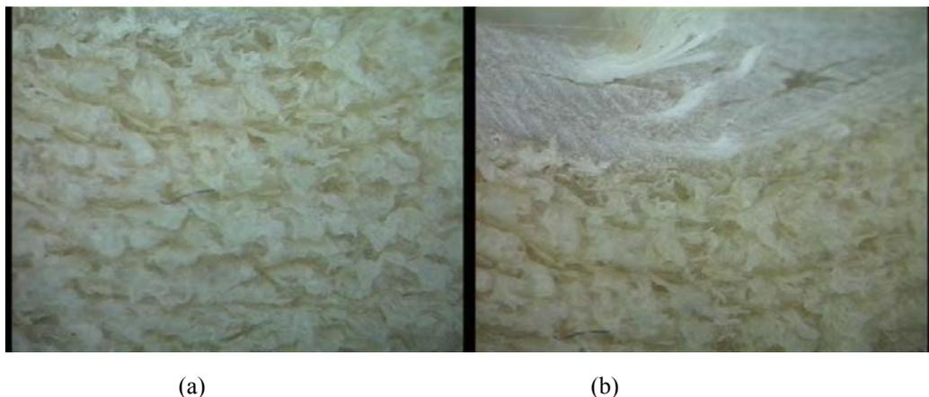
Fig.7. (a) Bands of collapsed of cells in HD core after  $10^6$  fatigue cycles at RT.  $P=0.65P_{ult}$ ,  $R=0.1$ ,  $f=3Hz$ , (b) Matrix cracking, fiber breakage and delamination on the upper face sheet of HD sandwich after  $10^6$  cycles at RT.  $R=0.1$ ,  $f=3Hz$ .
