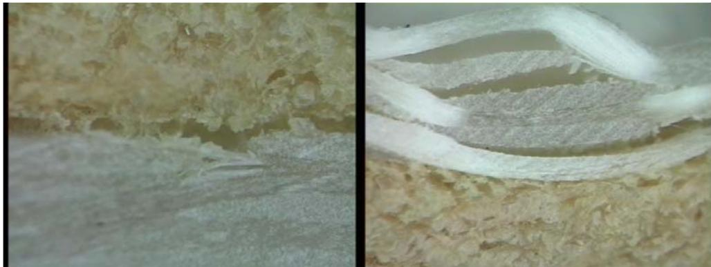
**Fig.9.** (a-b) HD sandwich beams after  $10^6$  cycles at 80°C (a) face /core delamination (b) delamination of face sheets at point of loading.
