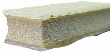
**Fig.8.** Degradation of HD core after  $5 \times 10^3$  cycles at 80 deg.C. The core concaved and the height of the beam reduced.
