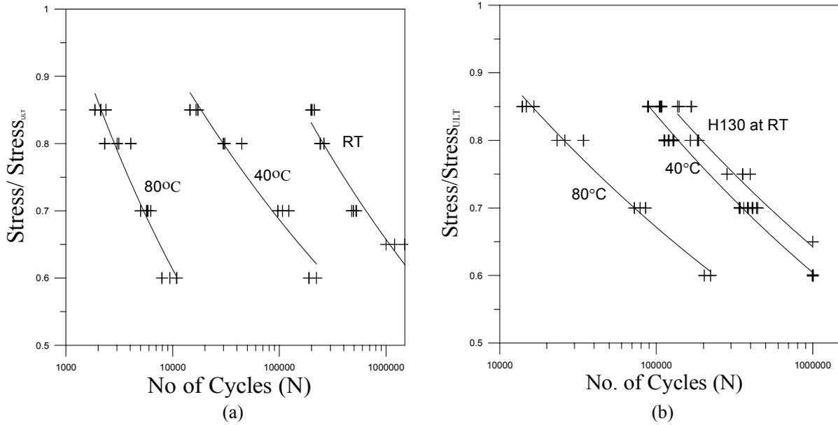
Fig.6. S-N curves at RT, 40 and 80°C for (a) HD sandwich beams and (b) H sandwich beams
