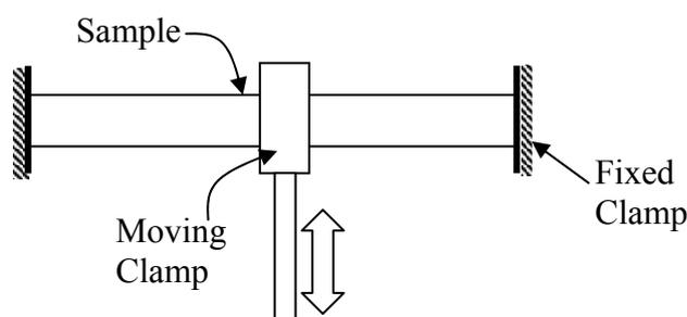
Fig.1. Schematic of 3-point bend clamp used for DMTA of HD and H foams
