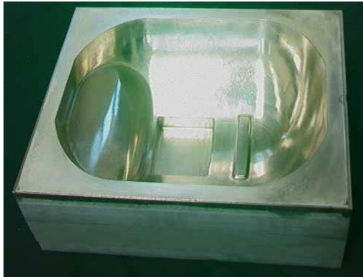
Fig. 10. Finished nickel mould
