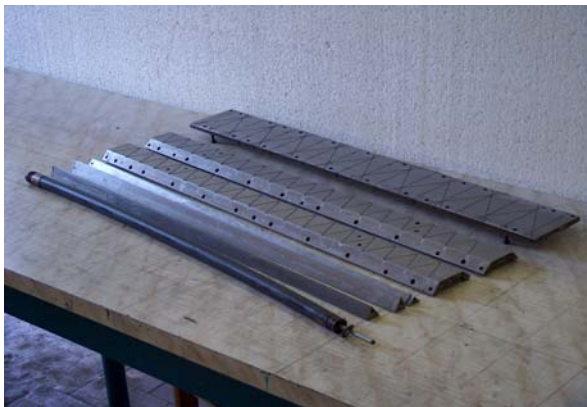
Fig.6 Components of the mould used for manufacturing the space frames.
