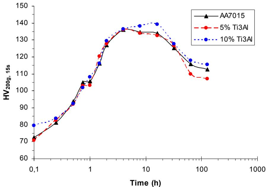
**Figure 7.** Vickers hardness evolution against ageing time at 150°C for the extruded base alloy AA7015 and composites with 5 and 10% of reinforcement.
