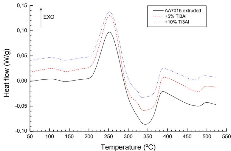
**Figure 6.** DSC runs of extruded AA7015 base alloy and composites reinforced with 5 and 10% of Ti<sub>3</sub>Al particles, after solution treatment at 480°C for one hour and quenched in water. Heating rate 20°C/min.
