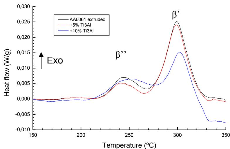
**Figure 2.** DSC runs of base alloy and related composite materials, after ageing 30 min. at 175°C from the “as quenched” condition. Heating rate: 20°C/min.
