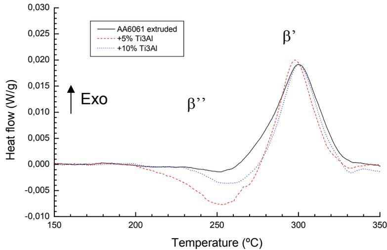
**Figure 3.** DSC runs of base alloy and related composite materials, after ageing 1 hour at 175°C from the “as quenched” condition. Heating rate: 20°C/min.
