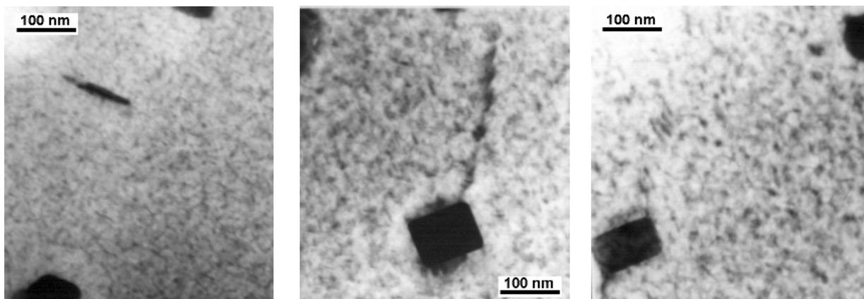
**Figure 5.** TEM Image of precipitates on AA6061 base alloy and related composites after 2 hours ageing at 175°C: a) extruded base alloy b) composite with 5%  $Ti_3Al$  c) composite with 10%  $Ti_3Al$ .
