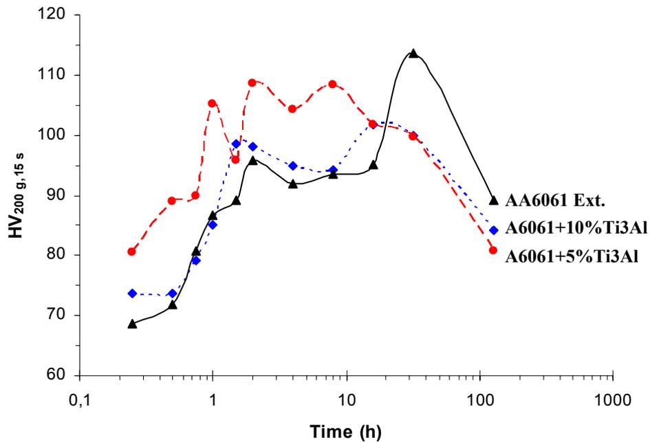
**Figure 4.** Vickers microhardness evolution for the different composites and the base alloy considered in this study. Solution heat treatment of 1 hour at 530°C, quenching in water and ageing at 175°C at different times.
