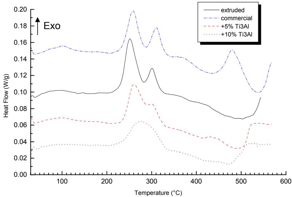
**Figure 1.** DSC plots of the materials studied after quenching in water. Heating rate: 20°C/min. Curves are displaced over y-axis for better display.
