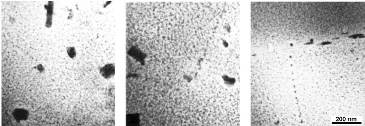
**Figure 8.** TEM Image of precipitates on A7015 base alloy and related composites after 8 hours ageing at 150°C: a) extruded base alloy b) composite with 5%  $Ti_3Al$  c) composite with 10%  $Ti_3Al$
