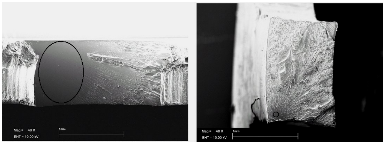
Figure 9. SEM pictures of BisEMA-5% OctaPOSS (left) and BisEMA-CHMA-5%OctaPOSS. The circles evidence the mirror zone
