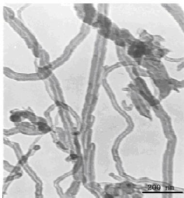
Fig.1 TEM image of carbon nanotubes powder before sintering
