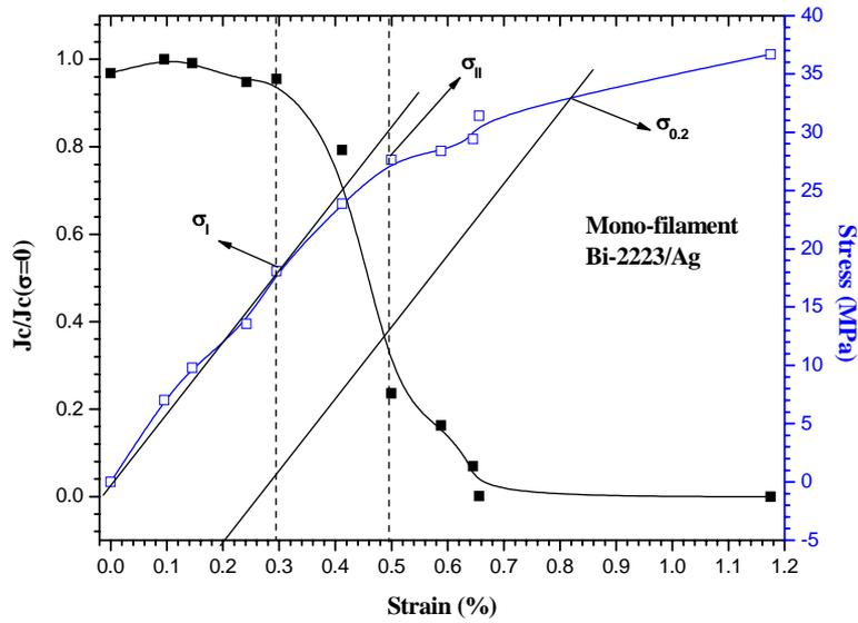
Fig. 5  $J_c/J_{c0}$ -strain-stress curve of monofilament Bi-2223/Ag tape
