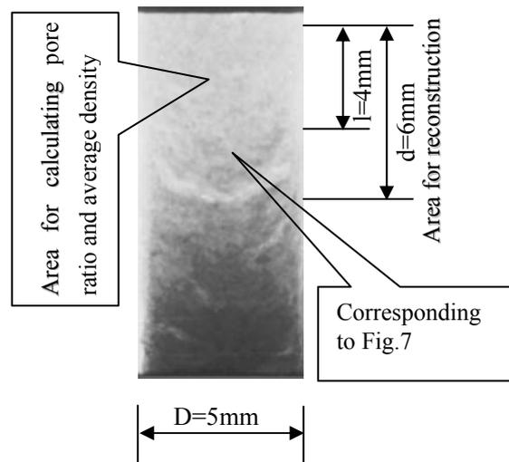
Fig.6 Projection slice at  $0^\circ$
