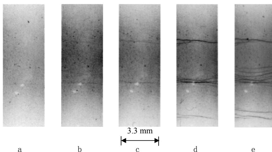
Fig.4 Damage evolution photographs of monofilament Bi-2223/Ag tape at 77K
