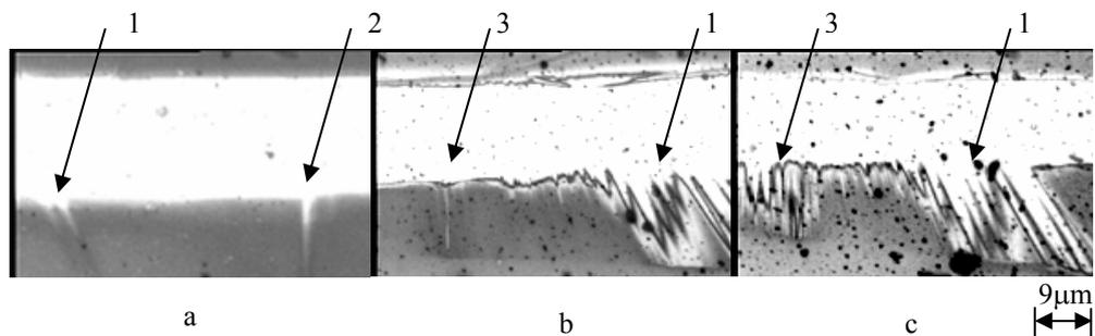
Fig.3 Damage evolution at interface between cover and fiber core
