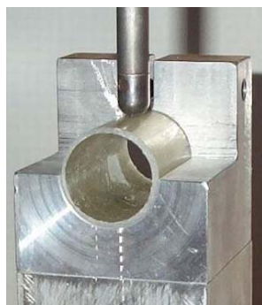
Fig. 3. Damage rig with tup and specimen
