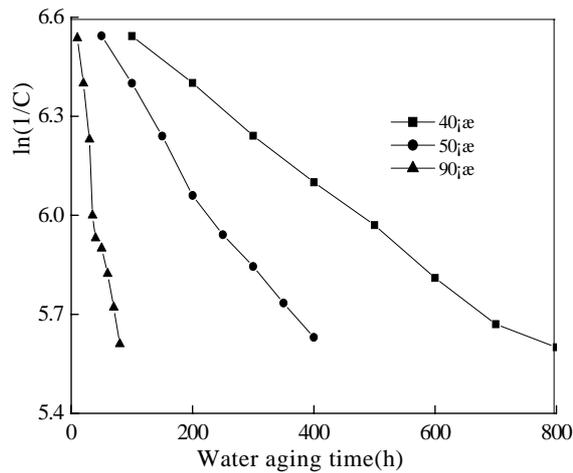
Fig. 5  $\ln(1/C)$  against water aging time of the joints treated by sand paper burnishing
