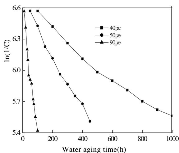
Fig.4  $\ln(1/C)$  against water aging time of the joints treated by chemical oxidation
