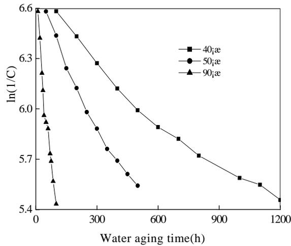
Fig.2 EDX analysis of  $\ln(1/C)$  against water aging time
