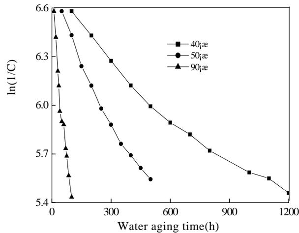
Fig.3 Elemental analysis of  $\ln(1/C)$  against water aging time
