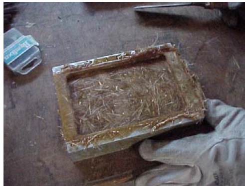
Fig. 4. Plate after the opening of the mould
