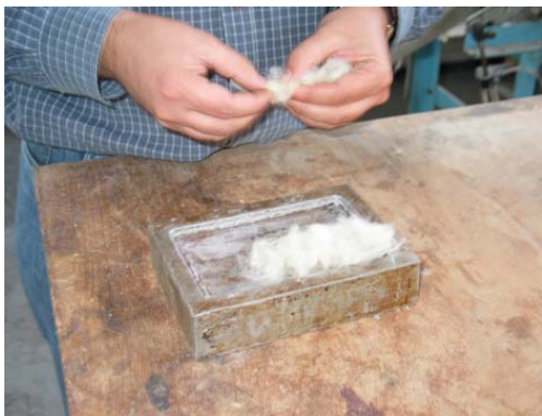
Fig. 1 - Lay up of the composite reinforced with tissue
