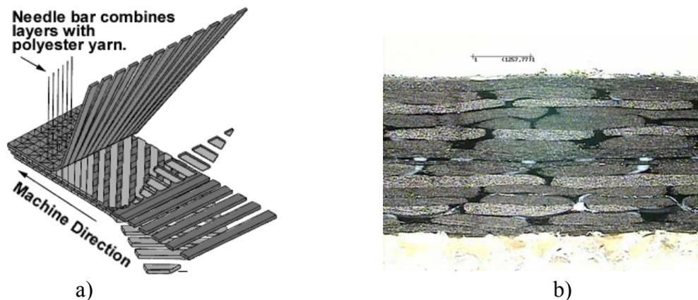
**Fig. 1.** a) Schematic of a NCF preform manufacturing (from Vectorply); and b) a cross section of quasi-isotropic NCF composite
