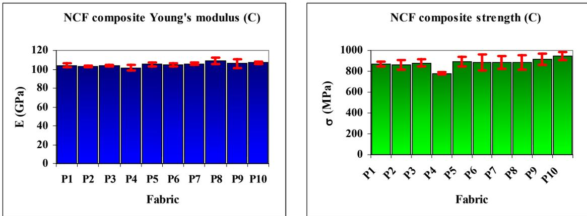
**Fig. 4.** Results from compression tests, scatter in data is indicated by scatter bars .
