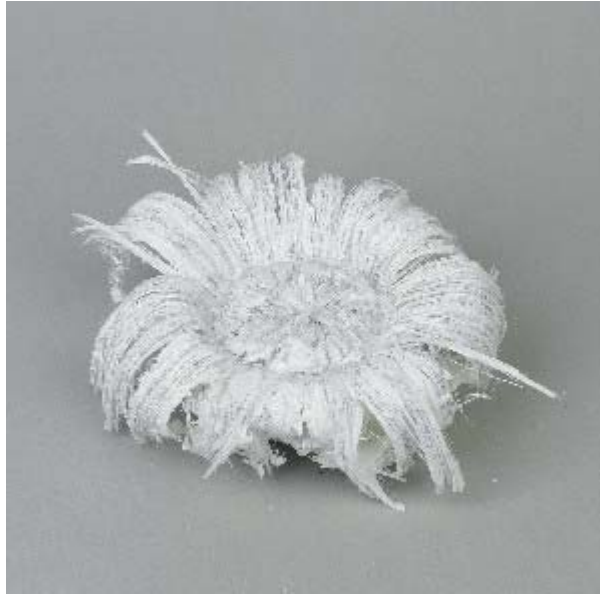
Fig. 3. Splaying/lamina bending crushing of a pultruded glass fibre-reinforced polyester tube.
