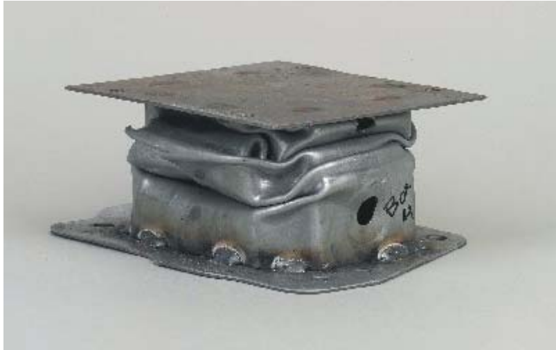
Fig. 1. Progressive folding of a steel crash box.
