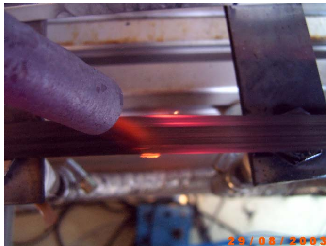
Fig. 8. Heating of thermoplastic tape material using hot gas.
