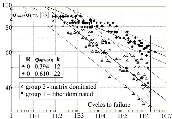
(a) Influence of the laminate behaviour for thermoplastic, carbon fibre, UD laminates at R=0
