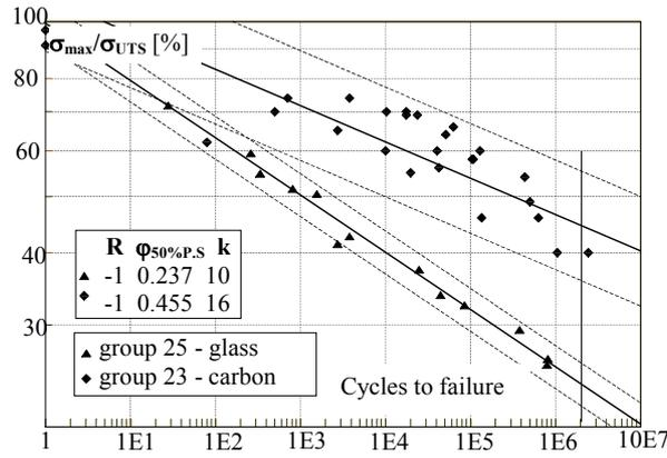
c) Influence of the type of reinforcement for thermosetting, fibre-dominated, woven laminates at R=-1
