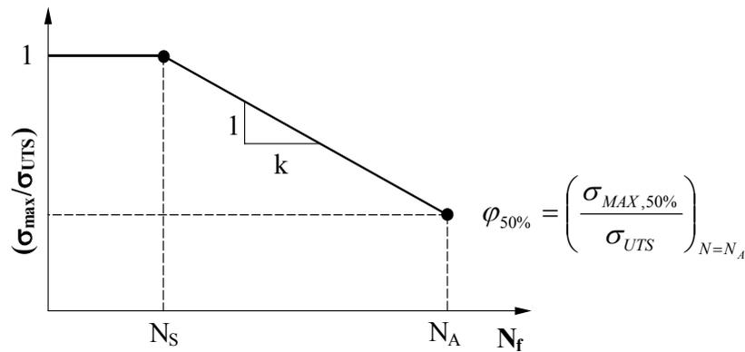
“Fig. 2. Normalised fatigue curve.”
