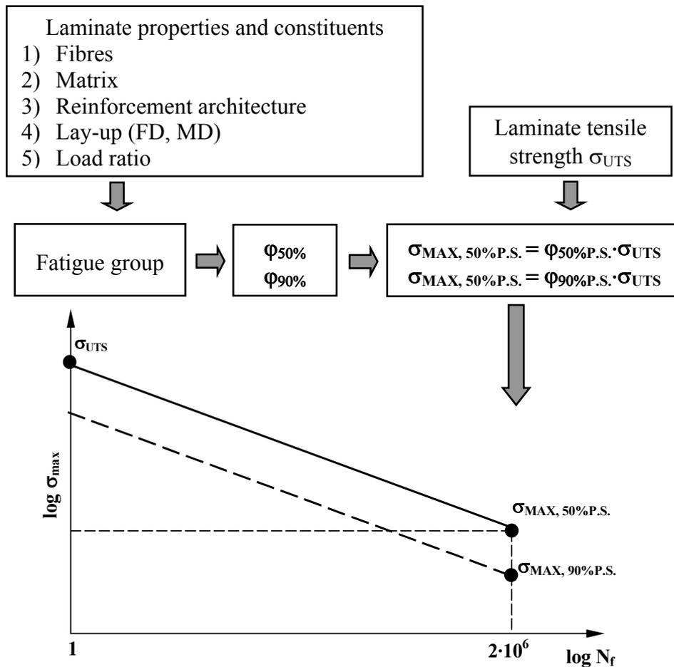
“Fig.4. Procedure for the construction of the fatigue curve of a generic laminate.”
