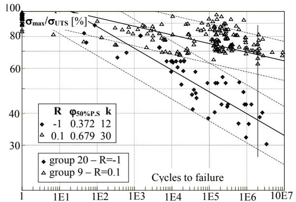
(b) Influence of the load ratio R for thermosetting, fibre-dominated, carbon fibre, UD laminates
