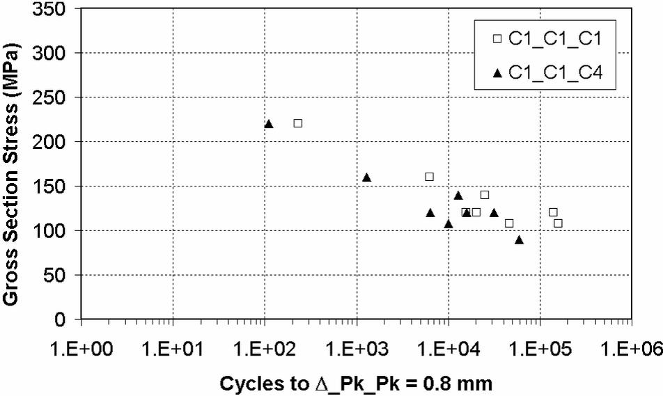
**Figure 6** Single-lap joints - cycles to “Hole elongation failure”, i.e. increase in peak-to-peak displacement of 0.8 mm
