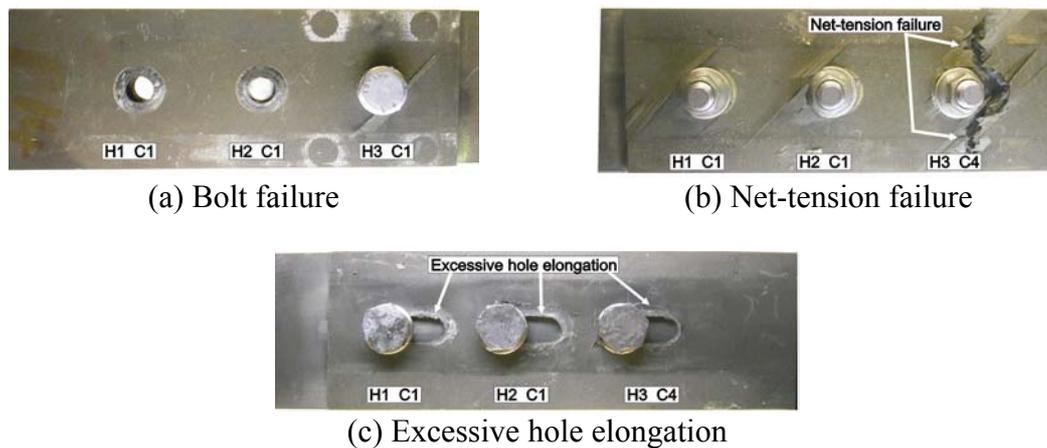
**Figure 5** Examples of the ultimate failure modes in the single-lap joints; double-lap joints exhibited hole elongation only
