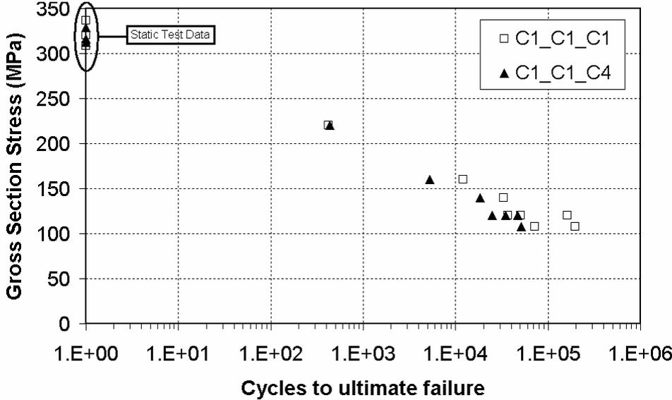
**Figure 7** Single-lap joints - cycles to ultimate failure
