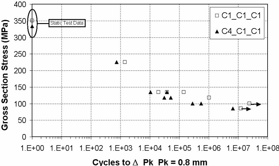
**Figure 9** Double-lap joints - cycles to “Hole elongation failure”, i.e. increase in peak-to-peak displacement of 0.8 mm. NOTE: Arrows indicate RUN-OUT, i.e. 0.8mm peak-to-peak increase was not reached
