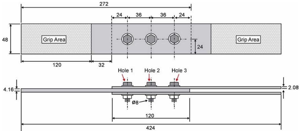
**Figure 2** Double-lap specimen geometry with hole numbering (all dimensions in mm)
