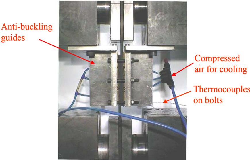
**Figure 4** Test set-up for fatigue tests (showing single-shear specimen)
