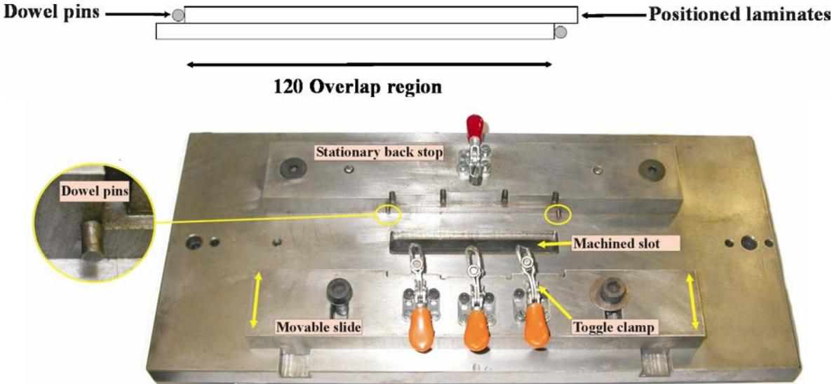
**Figure 3** Multi-bolt joint drilling jig (single-lap version)
