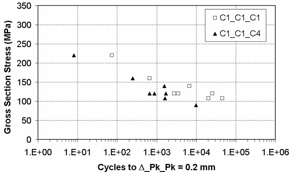
**Figure 8** Single-lap joints - cycles to an increase in peak-to-peak displacement of 0.2 mm
