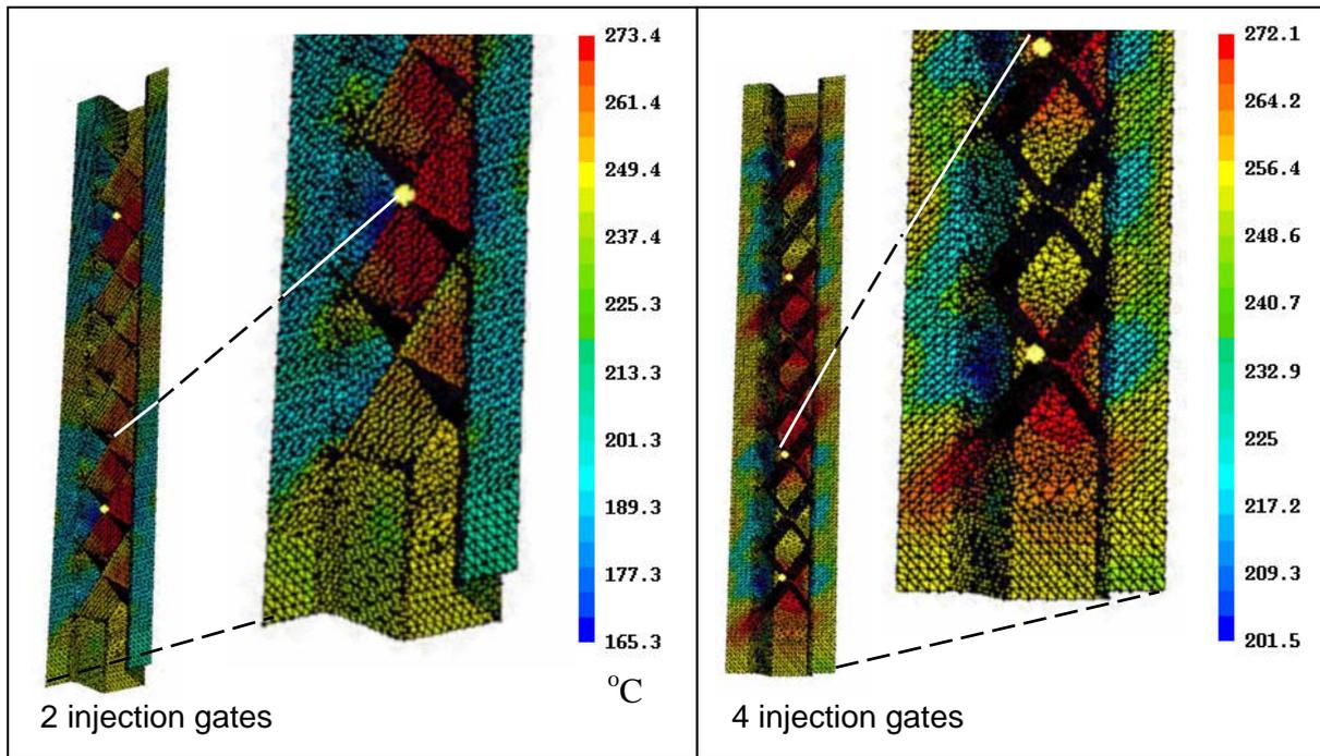
Figure 4 MoldFlow predicted temperature variations at 100% tool fill for: a) 2 injection gates, and b) 4 injection gates (*note separate temperature scales*)
