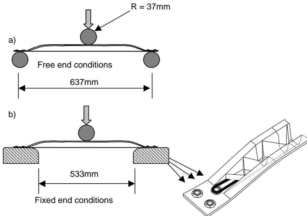
Figure 6 Beam testing: a) free-free end conditions, b) fixed-fixed end conditions
