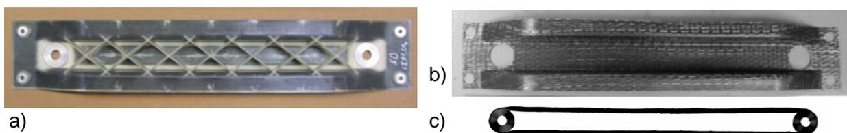
Figure 5 Hybrid beam and inserts
