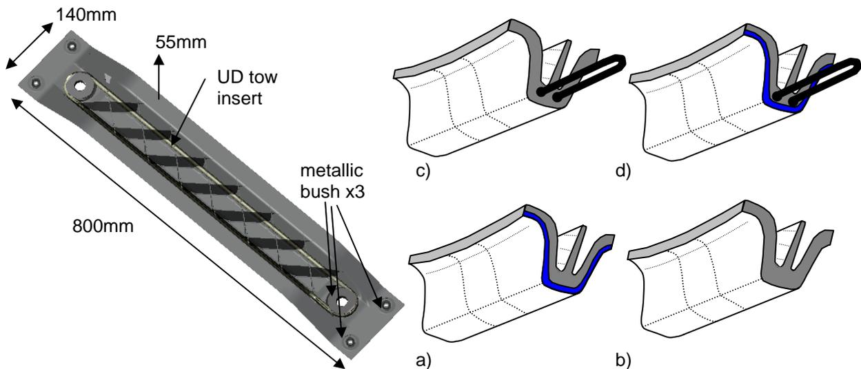
Figure 2 Generic beam tool geometry and cross-sections:
