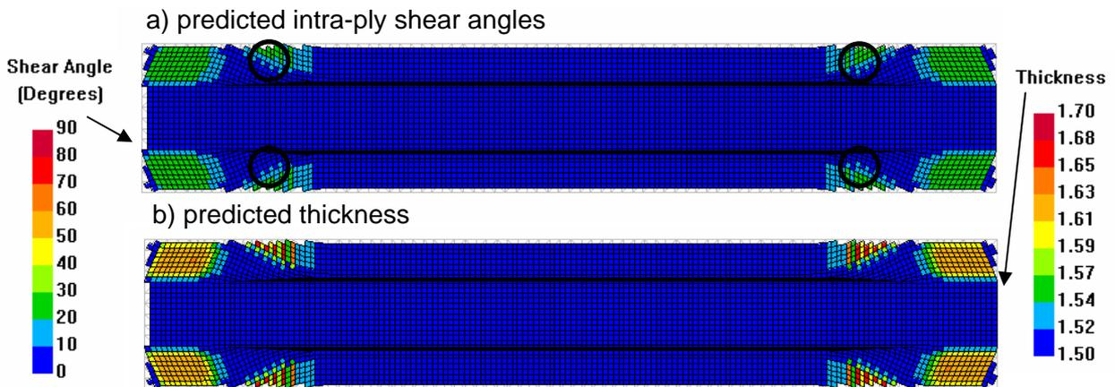
Figure 3 a) Predicted intra-ply shear angles for beam draped at 0/90°. The maximum shear angle is 28 degrees (circled).
