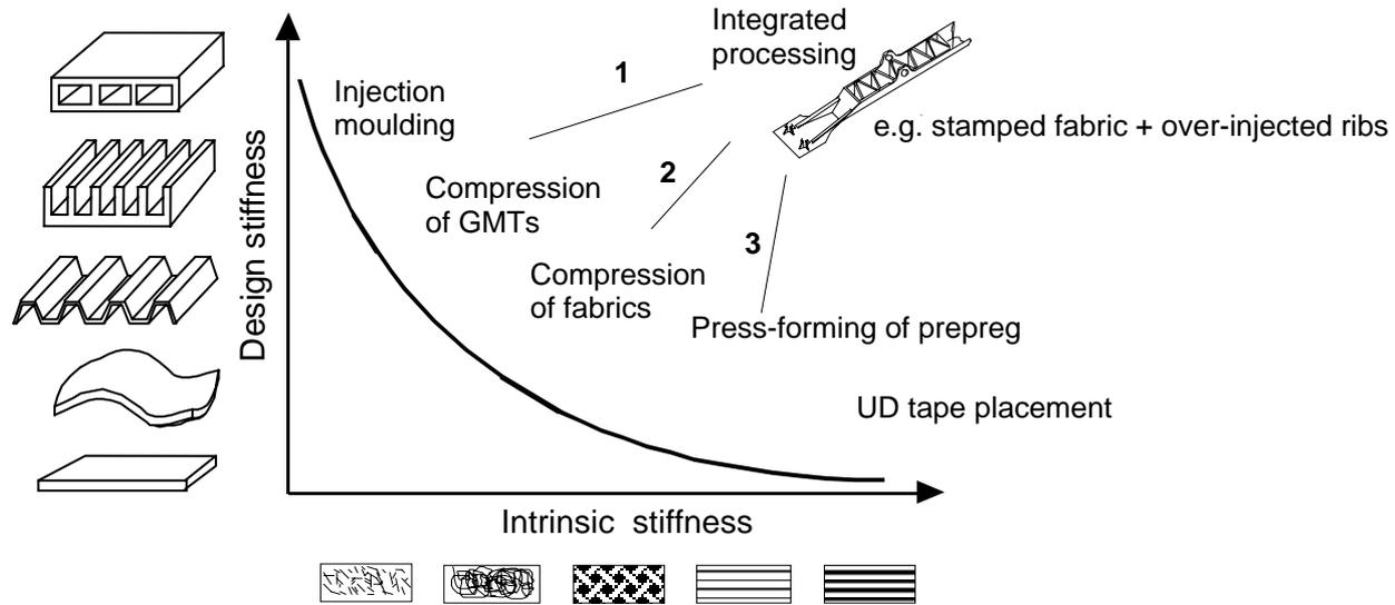
Figure 1 Combination of intrinsic and design stiffness via integration of multiple material forms and processing techniques
