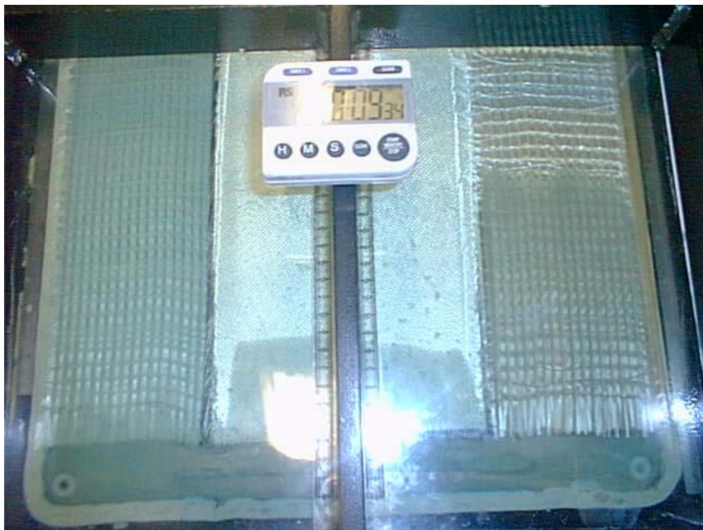
“Fig. 3. Flow progress in three parallel assemblies in an in-plane permeability RTM experiment.”
