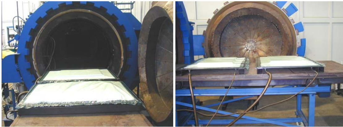
Fig. 2: Figure 1: High temperature autoclave
