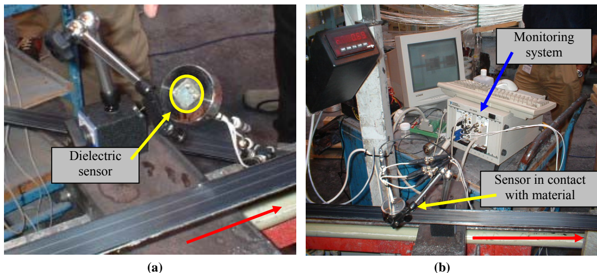
Fig. 7. Dielectric cure monitoring for pultrusion. (a) Sensor configuration, (b) Real – time monitoring system developed by INASCO Hellas [9]. The red arrows note the direction of movement of the pultrusion line
