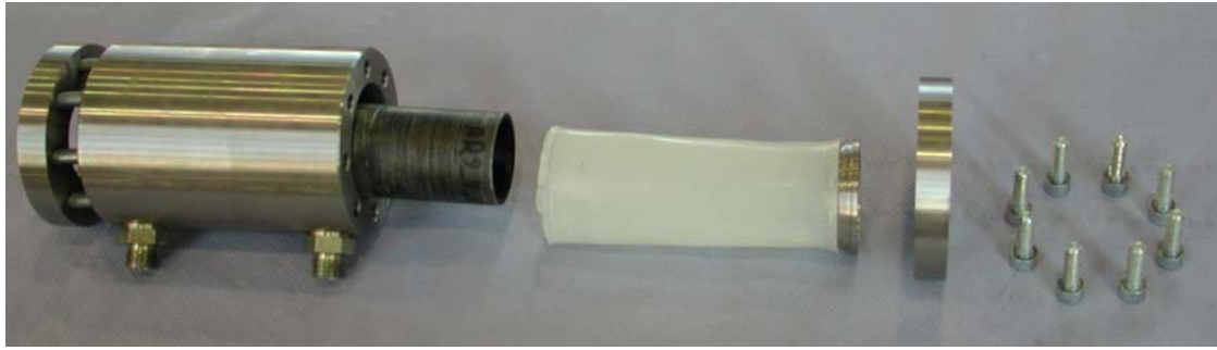
“Fig. 6. Test setup for biaxial compression loading.”
