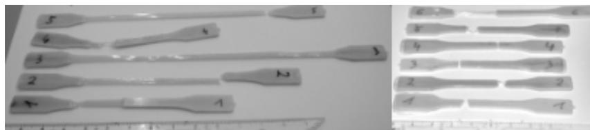
**Fig. 4 Tensile samples after testing (left) RP-PBT (right) RP-pCBT**
