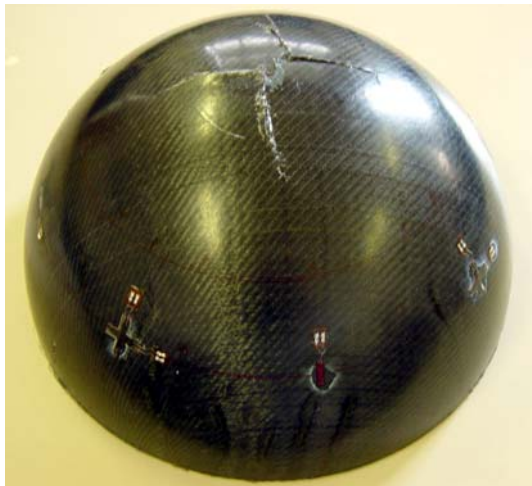
Figure 7 Top left: fracture on a big hemisphere; Top right: A compressed small hemisphere; Bottom right: Load set-up of the mudguard. A: The support plate; B: strain gauge; C: gluing the part on the support plate; D: The load head. Note deformations at the points C
