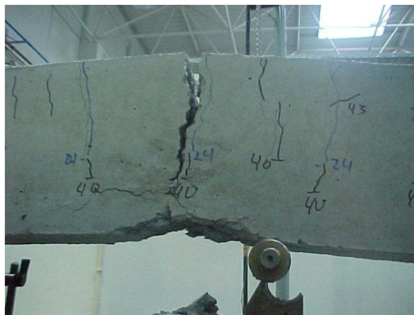
Fig. 7. Rupture of a reference beam.
