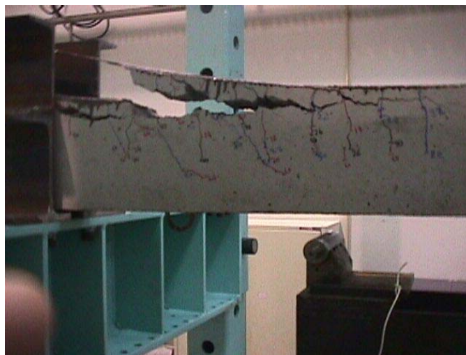
Fig. 9. Rupture of the reinforced beam
