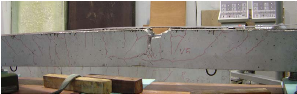
Fig. 10. Fatigue rupture of the reinforced beam (20%-70% máx load)
