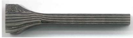
Fig.2. Cross section of the maximum loaded area with layer waviness and resin pockets
